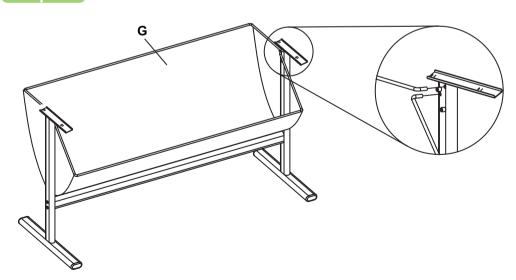
※ Note: Not to fully tighten the screws before well assembling the trimmer onto the stand.
