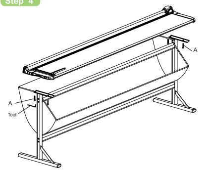
X Note: Not to fully tighten the screws before well assembling the trimmer onto the stand.
